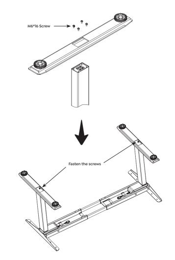
**Step 3:** Line up the screw holes on the feet and columns. Fasten the screws.
