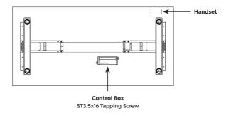
**Step 6:** As shown in the below, connect related parts, including control box, handset, extension cable and power cord etc. and fasten with cable clip.
