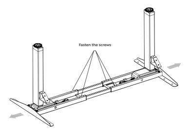
Avoid excessive tightening of screws. Both sides of the desk must be adjusted to the same width. The frame width is adjustable: 1100 - 1800mm, which is suitable for different desktops.
