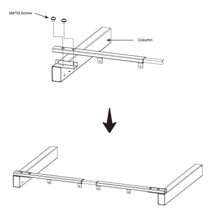
Avoid excessive tightening of screws
