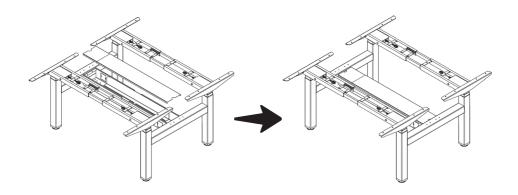
**Step 6:** Installing screen - fix chosen screens brackets (purchased separately) to the horizontal side rails and fasten the screws.
