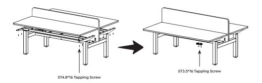
**Step 9:** Install control boxes on underneath of desktop (see below diagram). Control boxes must be installed flush and away from desk frame.
